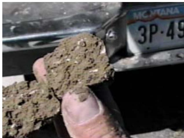
PHOTOGRAPH NO. 2 White spots indicate water percolating through soil at 6-foot level.
